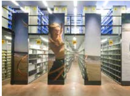
Multi-tier shelving with an integrated mezzanine floor is ideal when a large picking area is required, with limited floor space.
