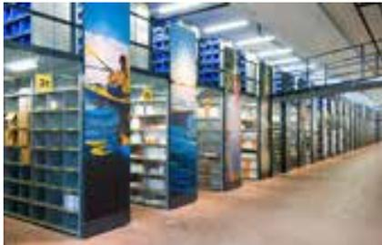
Smith & Nephew needed a new solution for their goods and associated packaging material. A Multi-Tier shelving systems was installed to support their European logistics operation for finished goods. For the storage of semi-manufactured products a Mezzanine floor was installed to create additional capacity.
